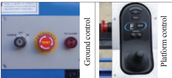
Emergency stop buttons / Tilt alarm
